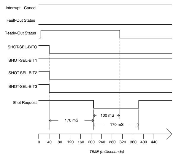
Fig. 34: External Control Timing Diagram
